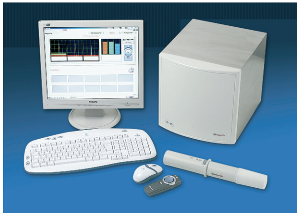
Figure 1. The TRIMprob system is composed of the exploratory probe, the receiver (a spectrum analyzer), and a laptop computer with dedicated software to manage patient information and store TRIMprob data.
